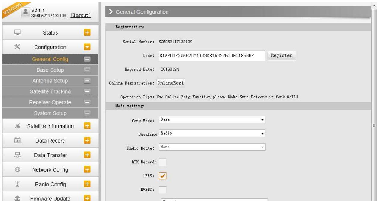
If the code of G6 has expired or is going to be run out, please provide the serial number of your G6 for us to apply for another available code, then input the code into the blank or register the receiver online.
