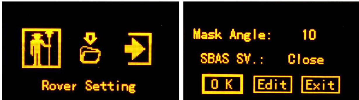
**Mask Angle:** It is an altitude restricted angle which is an angle defined from horizontal level to the sky direction, it is mainly used to control satellite view for GPS receiver. 10-15 degree is the default setting.
