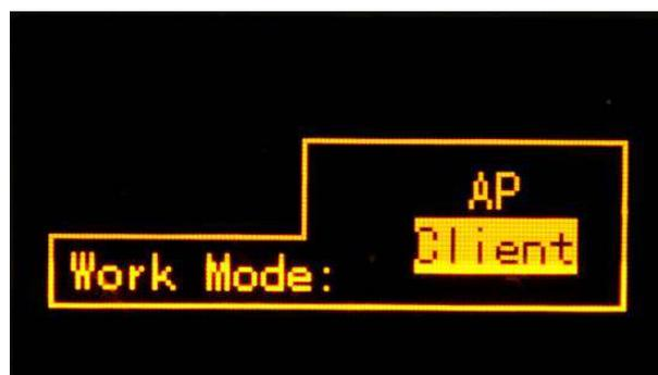
**AP:** This item means the WIFI hotspot broadcasted by G6 for mobile terminals such as smartphone or tablet to connect and access the Web UI.
