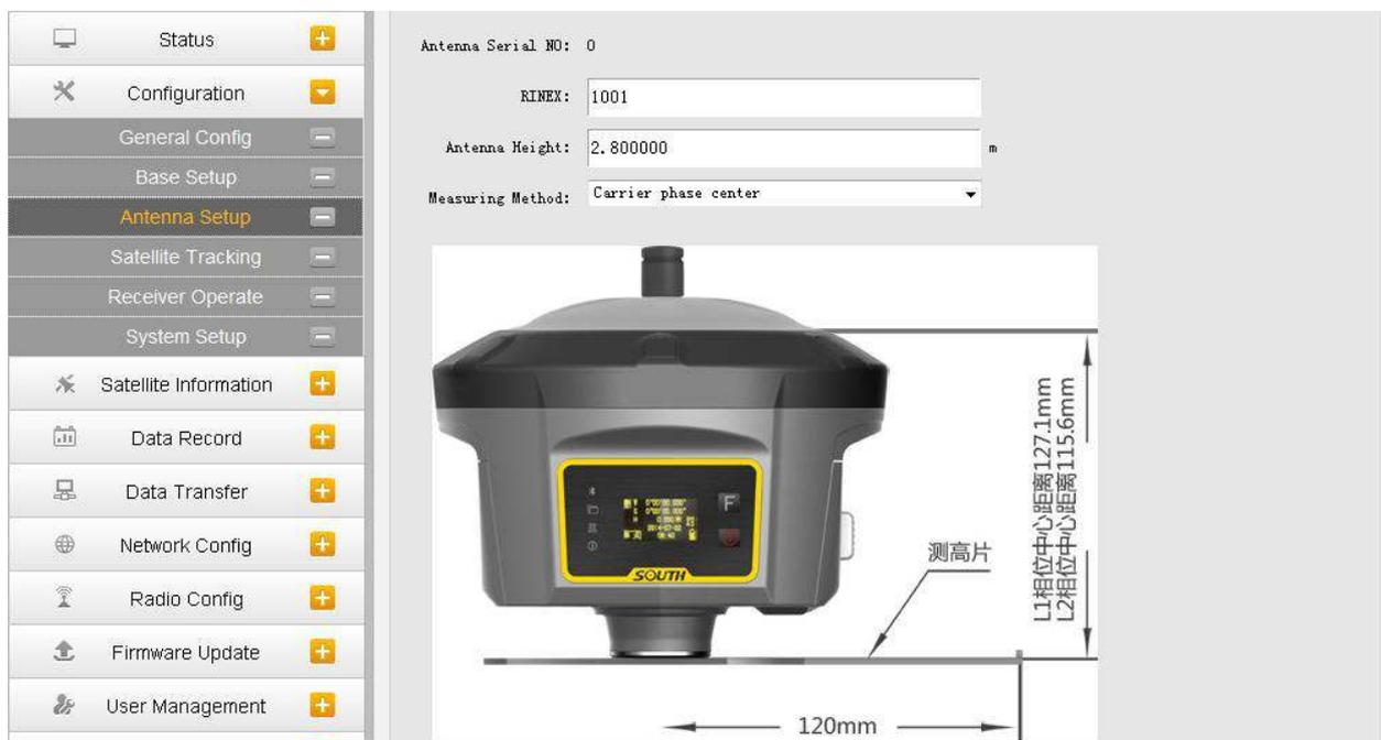
**Antenna Height:** This is the value for height of antenna while surveying.
