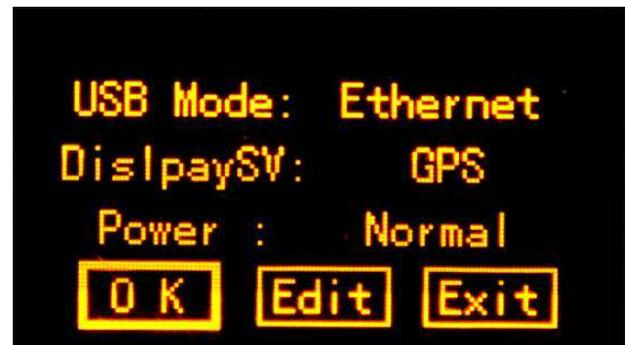
**USB Mode:** This is used to configure G6 what kind of mode output from 7-pin port when connect the receiver with computer via USB cable.
