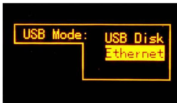
If **USB Disk** option is selected, then Galaxy G6 will be detected as a flash disk when connects to computer via USB cable, in this case, you can copy the static data from G6's memory folder.
