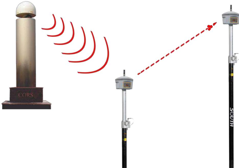
**RTK Record:** This is used to enable raw data recording in base mode or rover mode for post-processing
