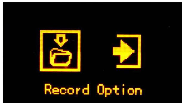
What we should do in the next is setup all the parameters for static mode. Press power key once and enter Record Option page, all the parameter items are displayed here including point name, antenna height, sample interval, record mode and data type.
