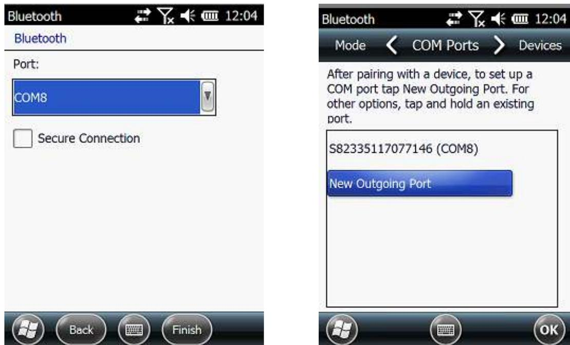
After the establishment of the virtual serial port, other applications can use the serial port for data communication with a Bluetooth device.
