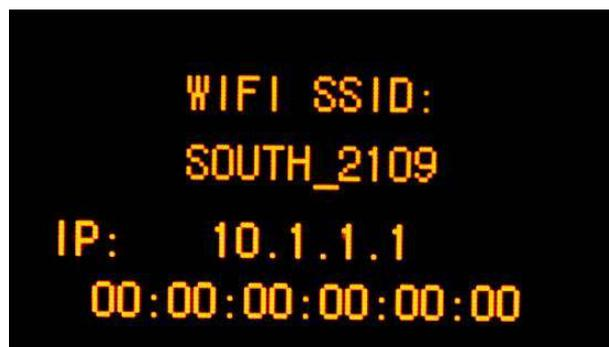
Search the WIFI SSID broadcasted by G6 with smartphone or laptop and connect it, then input the IP address 10.1.1.1 into the address bar of explorer and access to the web UI of G6.
