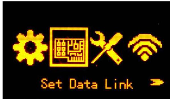
Press F key to get into main configuration interface after the initialization or the working mode has been setup, then move the select box to Set Data Link option by pressing F key, and press power key to confirm and enter the interface, there are UHF, Cellular Net, Bluetooth, Dual Transmitting, WIFI Datalink, External, Close Datalink and Main menu options displayed on this interface.
