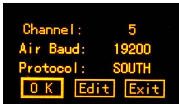
**Channel:** This is the communication channels for internal UHF, the value of the channel must be the same both in Base and Rover.
